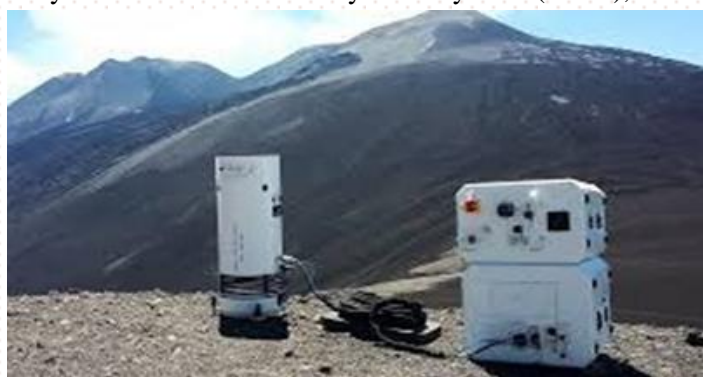
Fig 7: Quantum Gravimeter Source: Exail
