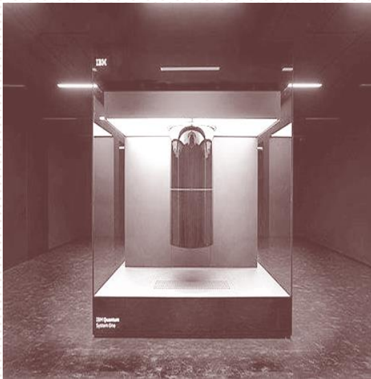
Fig 11: A quantum computer by IBM from 2019 with 20 superconducting qubits.
